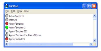
In the main window there is the list of hooked programs: DxWnd can currently handle up to 256. Trying to add more than that will give an error message. Keep in mind that DxWnd bundles usually contain an example configuration files with some entries already set, but because of the program absolute path value, chances are that none of the existing entries will actually work without some corrections.
